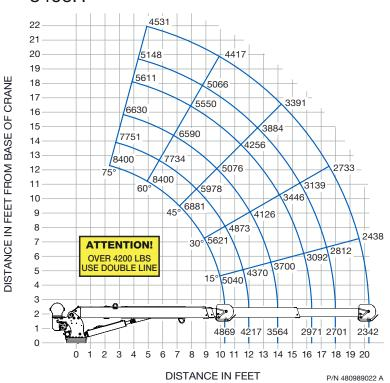
Note: Weight of load handling devices are part of the load and must be deducted from the capacity.
