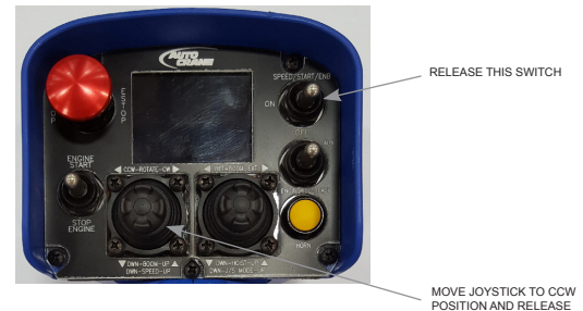
Figure 3—LCD screen display & transmitter during step 3
