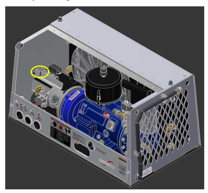
3. Identify the required wires in the harness that must be modified. A relay socket containing four wires is mated to the timer relay. Inspect this socket and verify that an orange 16 gauge wire is located in the 30 position of the socket and a white 16 gauge wire located in the 87 position of the socket. The two wires are circled in yellow in the image below.
